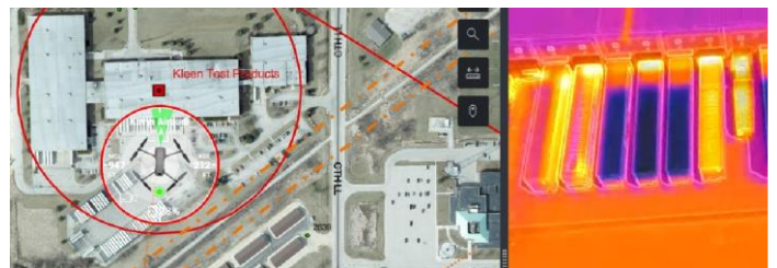
Above: Chemical facility showing buffer zones for each chemical stored on site and thermal imaging of storage trailers.
